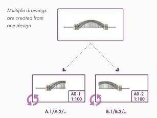
The relationship between a CAD file and its references is stored within the CAD file (e.g. AutoCAD, MicroStation), and sometimes additional references are stored in an external file (e.g. project file) or database (e.g. ADT, Civil 3D, Inventor). This means that an engineering document management system will only manage CAD files properly if it is able to "read" the reference information and if it is integrated deeply with the CAD application used to create and edit the CAD files.
